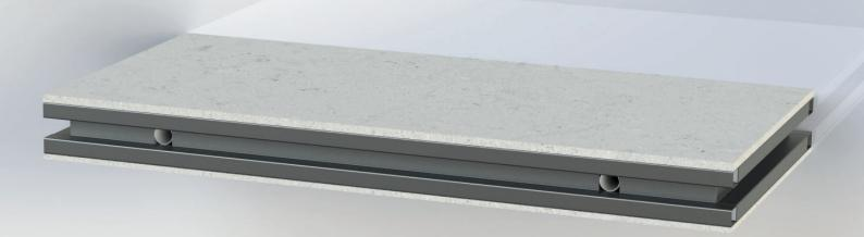
Structural Insulated Panel, used as external wall of PANHOUSE system. It has an external cladding in Magnesium Oxide, an excellent inorganic fireproof and waterproof material, and a core made of EPS or Mineral Wool. The panel is made with perimeter structural steel, which give resistance up to 75.0 psi, as per Florida Building Code (2014) TAS 202. The panel is pre-set internally for technical equipment (electricity, water and gas); it can be painted or coated.
